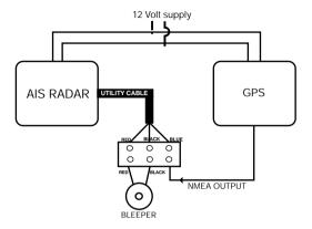
Connect the NMEA output (or NMEA +) of the GPS to the BLUE wire of the UTILITY cable. If the GPS has a NMEA - or NMEA REF connect this wire to the vessel supply negative. The AIS radar requires an NMEA 0183 signal with RMC sentence. The signal15.059
